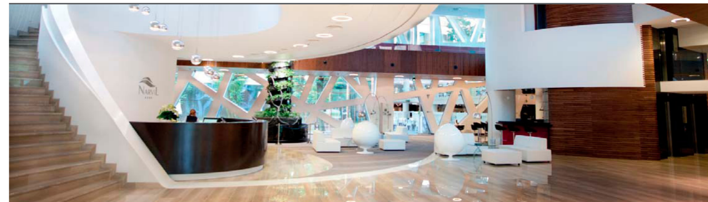
Hotel lobby with a view to the main reception and to the bar. The reception desk is made of wood-based materials, with the use of Staron-type conglomerate. The lobby walls are covered with veneered cladding in nut-brown color. Stand-alone upholstered furniture pieces are covered with fire-retardant fabrics.
